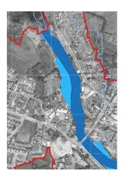
Ballysadare - floodinfo, 1% and 0.1% AEP flood extents
